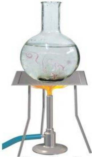
Convection of heat in water
