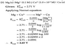
Discussion of various problems and case studies.for example Effect of external voltage on direction of current in a electrochemical cell as shown below-
